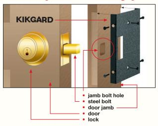
Conventional door-locking systems send a steel bolt through a small hole in wooden doorjambs only 1/2" from the edge of the jamb. Without effective reinforcement, all that an intruder needs to break to enter a home is that 1/2" of soft wood.
